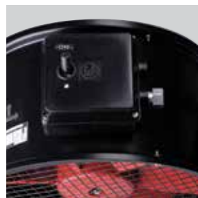
Flame retardant terminal box Wiring terminal box in flame retardant plastic V0 fixed to the exterior of the casing and provided with a two-pole On/Off switch. Cable gland PG-11.
